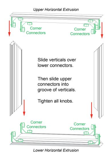
Adjust connectors if necessary to prevent gaps in connection.
